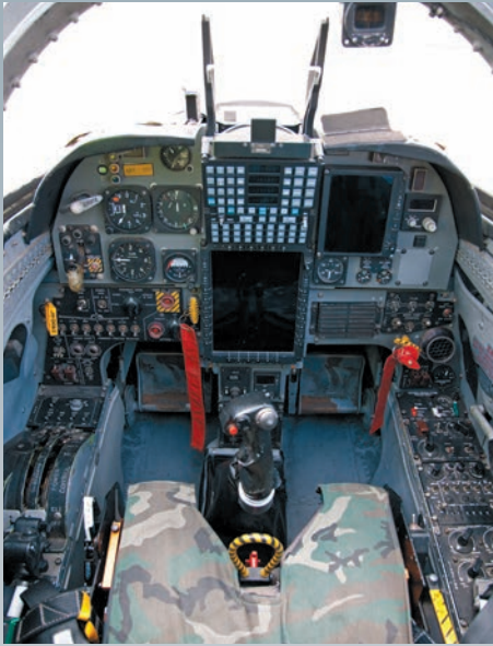
Above: The 'office' of the F-5M is fitted with two large multi-function displays that replaced the old analog versions during the upgrade program.
